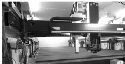
The robotic freezer can store over 3 million samples at -80°C. Any individual tube can be automatically accessed from anywhere within the 10 different freezer compartments.
